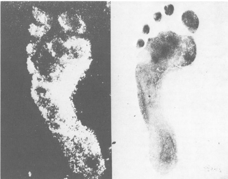
FIG. 15— Comparison of the pattern of a bare left foot disclosed by luminol at the residence of a missing person and the inked impression of the left foot of a suspect.
